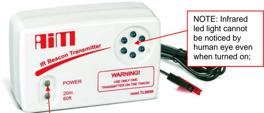
**NOTE:** Infrared led light cannot be noticed by human eye even when turned on;
