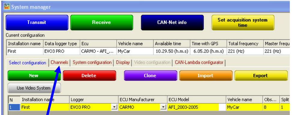
Activate “Channels” layer. It allows you setting the channels acquired by EVO3 and its layout depends on EVO3 version.
